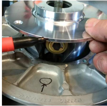
13) Install the T25 screws to hold the helix using a drop of blue thread locker. (48 in./lbs.)
