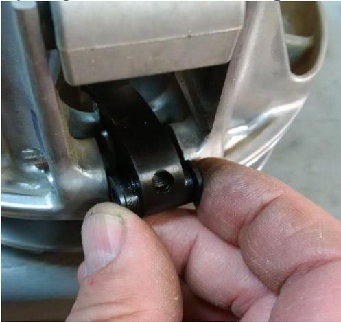
With stock clutches it is very common to see the side of the clutch wearing from the flyweight pivot end gouging into the aluminum, even with only low miles.
